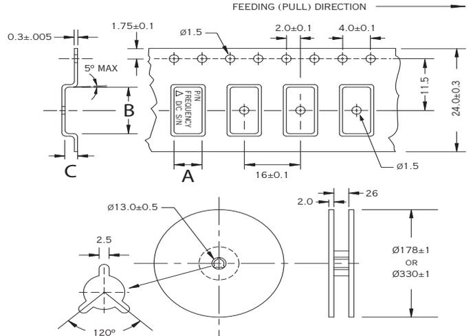
Dimensions are in mm. Tape is compliant to EIA-481-A.
