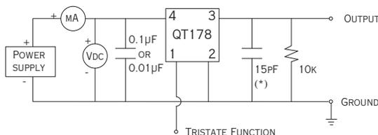
(\*) CL INCLUDES PROBE AND JIG CAPACITANCE
