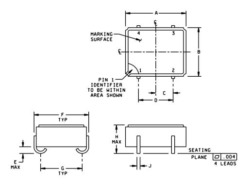
FIGURE 1. Interface and physical dimensions.
