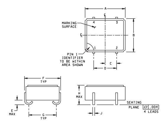
FIGURE 1. Interface and physical dimensions.
