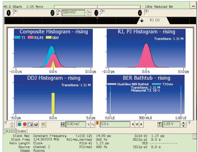
Figure 1: Jitter Analysis of a QT82LD-125MHZ
