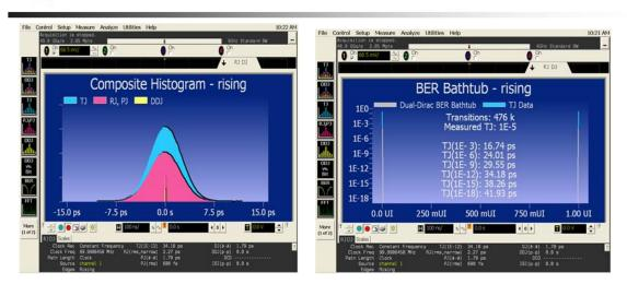
Deterministic jitter is <u>clock</u> timing jitter or data signal jitter that is predictable and reproducible. The peak-to-peak value of this jitter is bounded, and the bounds can easily be observed and predicted.
