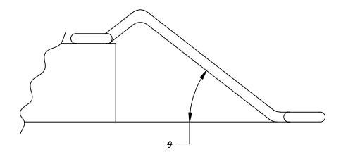
FIGURE 2023-1. Wire loop angle.
