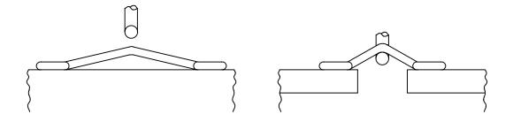
FIGURE 2023-2. Flat loop wire pull testing.
